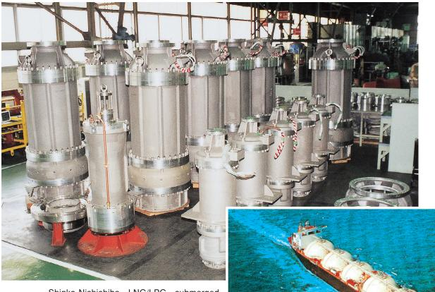
Shinko-Nishishiba LNG/LPG submerged motor pumps are used in many storage stations. And, the cargo pumps for LNG/LPG tankers are also installed on a large number of ships.
